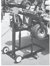
Mo-Jack's self-braking winch lifts the mower on a T-shaped lift bar that supports the front wheels.
