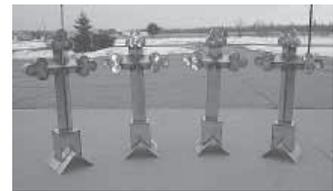
He used the press to make four church crosses out of stainless steel tubing.
