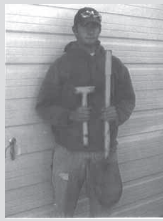
Dearden fashioned hammer out of pipe. He uses it on an old shovel with a length of pipe welded on in place of its missing handle.
