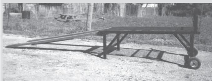
Service rack mounts on four 26-in. high legs. A pair of wooden ramps is attached to one side, and an 8-in. high metal bar acts as a "stop" on top.
