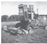
John Herren mounted his Brillion flail mower on an old Case combine. "The combine gives me variable speed on the drive wheels while maintaining high rpm's on the mower," he says.
