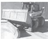
For blading work, a hydraulic cylinder is extended to angle the blade up to 31 1/2 degrees to one side.
