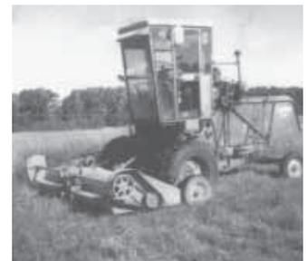
**John Herren mounted his Brillion flail mower on an old Case combine. "The combine gives me variable speed on the drive wheels while maintaining high rpm's on the mower," he says.**
