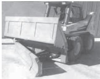
**For blading work, a hydraulic cylinder is extended to angle the blade up to 31 1/2 degrees to one side.**
