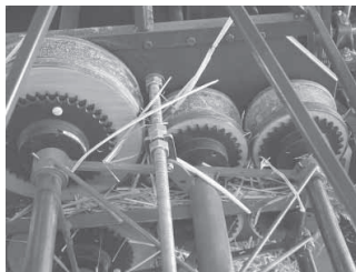
Strawjet machine makes tightly compressed, wrapped cables of straw from windrows in the field, above. Compression wheels, below left, pack the straw. Cables are “cemented” together with a clay-based adhesive and then plastered over, below right, to make beams and panels.
