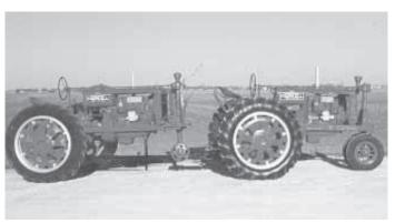
Daniel Lowe joined these Farmall F-20s together using a farmer-built hitch. Lever hooked to clutch of rear tractor extends up and over the hood.
