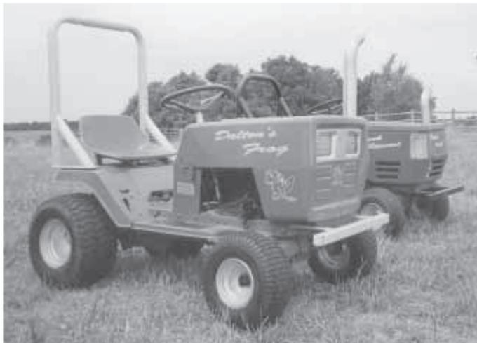
Tractors are fitted with rollbars and front bumpers. Original muffler was replaced with a 2-in. dia. tractor muffler, which is bent so exhaust fumes are diverted to the side.
