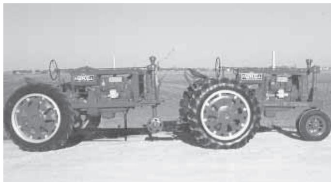
Daniel Lowe joined these Farmall F-20s together using a farmer-built hitch. Lever hooked to clutch of rear tractor extends up and over the hood.
