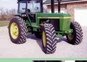
By replacing the spindles and outer part of the front axle on his Deere 4430 tractor with spindles off a Deere 7720 combine, Dennis Flanery was able to mount bigger tires. It gives the tractor better flotation on soft and rough ground.
