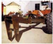
Two-wheeled, pull-type rock digger has a pair of hydraulically-pivoted, 40-in. long steel "teeth" spaced about 16 in. apart.
