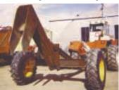
Machine's pivot arm is controlled by a 4in. dia. hydraulic cylinder.
