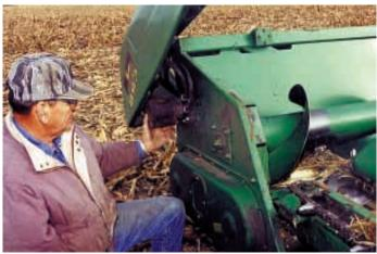
Litchfield bolted a hydraulic motor onto the header on his Deere 9650 STS combine. Motor which chain-drives auger runs off reel drive on grain head.
