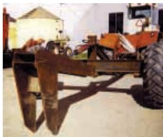
Two-wheeled, pull-type rock digger has a pair of hydraulically-pivoted, 40-in. long steel "teeth" spaced about 16 in. apart.
