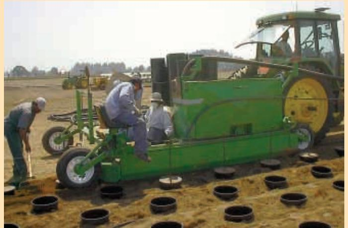
Pot-setting rig excavates a ditch where pot will be set and lays down a drain tile in bottom of ditch. Irrigation pipes are run alongside.
