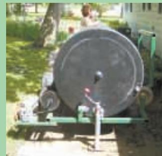
Barrel is powered by a 1/3 hp electric motor and spins about one revolution per minute.
