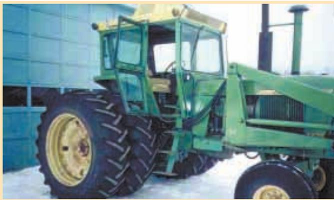
Meyer spent just \$50 and about half a day adding a second cab door to his Deere 4620. He says the idea would work on any older 20 series Deere cab.
