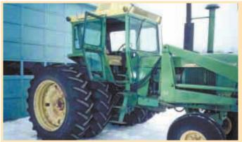
Meyer spent just \$50 and about half a day adding a second cab door to his Deere 4620. He says the idea would work on any older 20 series Deere cab.
