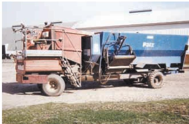
Mullenbach reworked a Patz 375 cu. ft. TMR mixer to build this self-propelled model.
