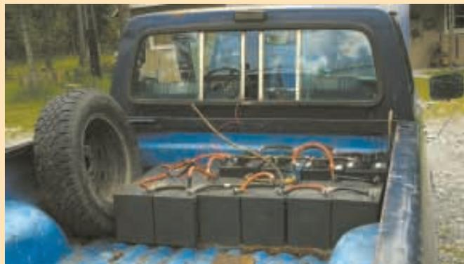
There are twelve 12-volt deep cycle batteries in the bed of the pickup.
