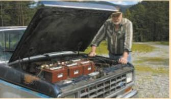
Bill Wilson converted his 1983 Ford Ranger pickup to electric power. Instead of an engine, the pickup now has six 6-volt, deep cycle batteries under the hood
