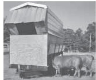
Home-built, weather-proof wagon doubles as a feeder. There's a hinged, 2-ft. high metal lid on each side of wagon at bottom.
