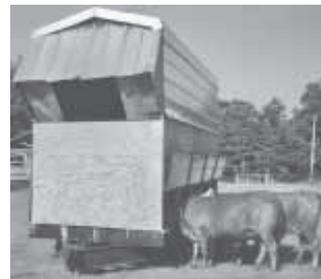
Home-built, weather-proof wagon doubles as a feeder. There's a hinged, 2-ft. high metal lid on each side of wagon at bottom.
