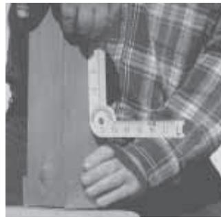
Folding multi-tool does the job of a level, square, bevel and ruler. Device is designed to "click" on the most commonly used mitre angles.
