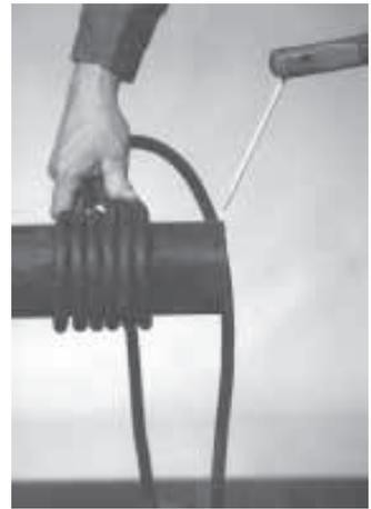
To neutralize strong magnetic fields, Galloway wraps lead wire around pipe before applying direct current.
