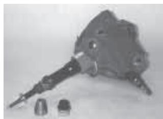
ering the cost of making holes, another advantage is speed. Holes are punched in one or two seconds. The tool works very well in ordinary sheet metal as well as aluminum.
