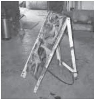
of front wheel drive cars. I bolted the fans in a fold-up angle iron frame. To operate the fans, I just hook them up to a vehicle's battery. I can operate either fan independently, or both together at the same time.
