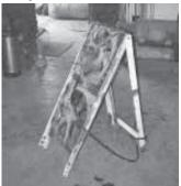
of front wheel drive cars. I bolted the fans in a fold-up angle iron frame. To operate the fans, I just hook them up to a vehicle's battery. I can operate either fan independently, or both together at the same time.
