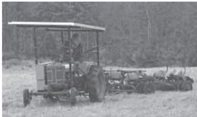
**John Howe's solar panel-equipped Cub Cadet can pull a 6-ft. harrow without burning an ounce of gas.**
