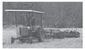
John Howe's solar panel-equipped Cub Cadet can pull a 6-ft. harrow without burning an ounce of gas.
