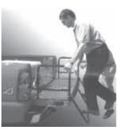
Kwik Gate step extends out over the tailgate. Back panel flips down to be used as a step.
