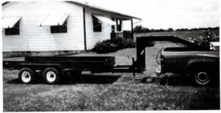
plywood wind deflector when pulling the travel trailer. It mounts on top of the gooseneck and has storage inside.
