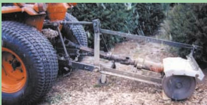
Manuel Escobar's 3-pt. mounted, pto-driven stump grinder is equipped with five 12-in. dia. cutting blades. They mount side by side on a 1-in. dia. shaft.
