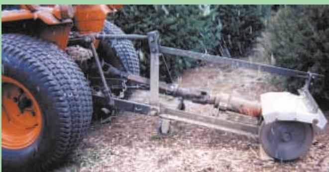
Manuel Escobar's 3-pt. mounted, pto-driven stump grinder is equipped with five 12-in. dia. cutting blades. They mount side by side on a 1-in. dia. shaft.
