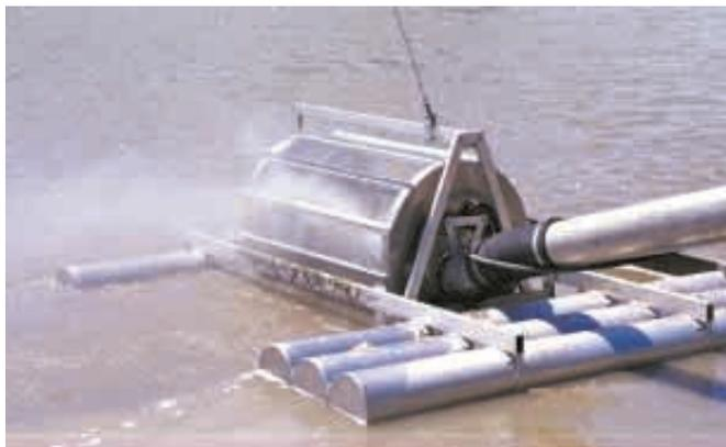
Water-driven, self-cleaning pump is designed to work in water as shallow as 4 in.
