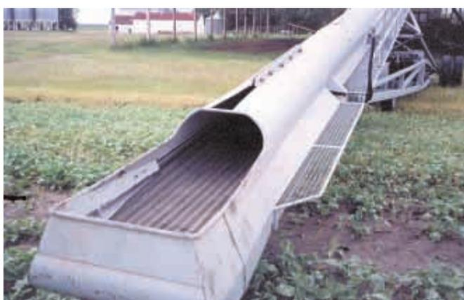
The Peterson brothers built this 100-ft. long, self-propelled grain conveyor from a 20-in. dia. steel tube and a 30-in. wide rubber belt.
