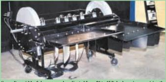
Spreading width of chopper can be adjusted from 20 to 45 ft. by lowering or raising the tailboard from 5° above horizontal to 35° below horizontal.
