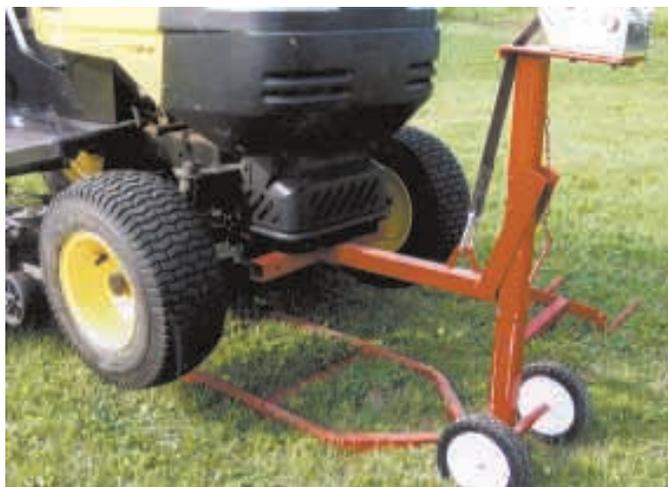
Fold-up portable jack is equipped with a self-braking winch. It lifts up to 350 lbs. on a T-shaped lift bar that supports mower's front wheels.
