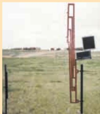
Gate lifts vertically out of the way so it's not hindered by obstacles such as snow drifts or livestock.
