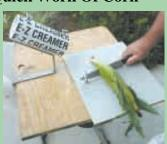
Cutting board and husking tube makes it easy to shuck the corn before creaming. Entire unit is made from plastic and stainless steel so it won't rust.
