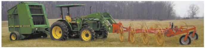
"Rake & Roll Hitch Kit" lets you rake and bale in one pass. Rake attaches to tractor's front-end loader.
