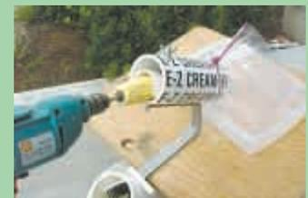
Once cob is screwed onto drill, husks and silk are removed by husking tube (at bottom in photo) and then the corn is “creamed” as shown in photo.
