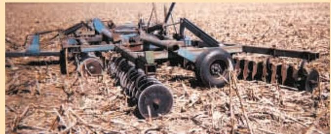
Mussman installed a row of straight coulters on front of disk and reversed the angled disk gangs on the back.
