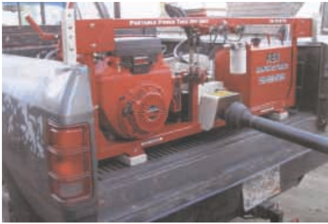
Portable power unit can be used on a pickup, trailer, or even as a stand-alone unit. It can be used for both pto and hydraulic work.
