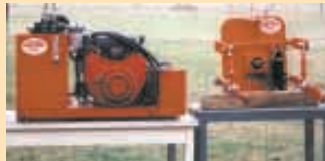
Power is supplied by a 24 hp Honda gas engine that drives a hydraulic pump. The pto and 3-pt. lift arms mount on a backing plate that fits into pickup's receiver hitch.
