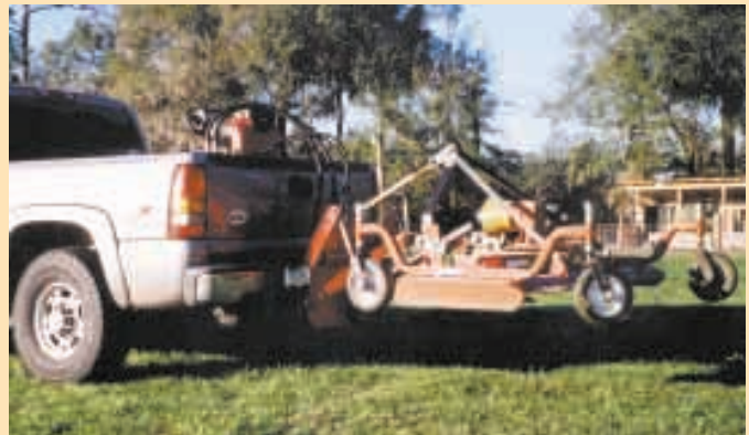
Pickup-mounted 3-pt. hitch has power up, power down, and draft control.
