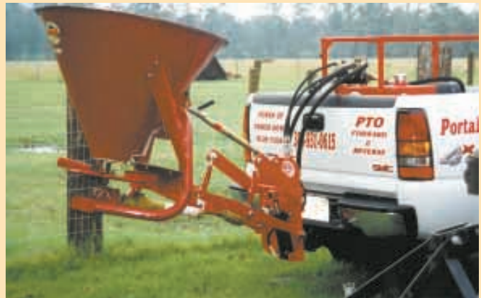
Portable 3-pt. hitch can operate attachments that would normally require a tractor.
