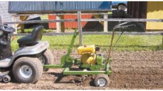
In the raised position, the rear wheels of the tiller are actually about 1 in. above the trailer wheels. At full depth all four wheels are at the same level.
