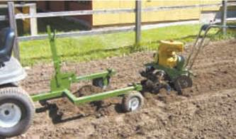
Rototiller pins to 2-wheel frame behind tractor. Depth is controlled by a lift lever on front
