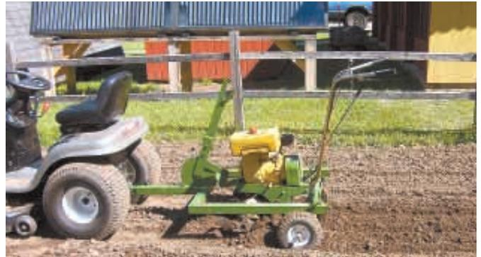
In the raised position, the rear wheels of the tiller are actually about 1 in. above the trailer wheels. At full depth all four wheels are at the same level.
