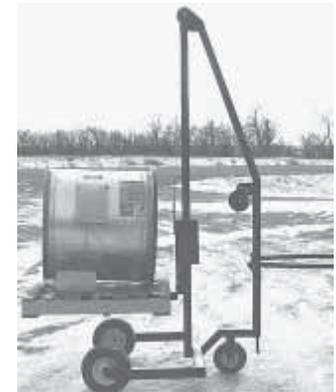
You can lift 500 lbs. to a height of up to 7 ft. with this hand-cranked lift.
