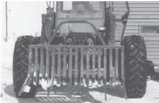
Smaller fork is 5 1/2 ft. wide by 5 ft. deep and has 17 tapered teeth spaced 2 in. apart. Teeth can be removed temporarily for certain jobs.
