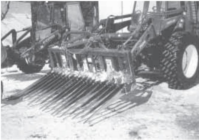
Fork is 9 ft. wide by 5 ft. deep and has 18, 5-ft. long tapered spears that are spaced about 6 in. apart.
