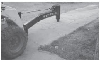
Hammer lifts by hydraulics and drops by gravity to strike with its 4 by 4-in. hardened tip. Very little vibration or shock load transfers back to the skid steer.
