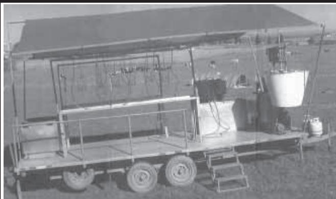
**Trailer rents for 30 cents per bird and includes propane. Comes with cones, scalding plucker, eviscerating table, final cleaning table and two chill tanks.**
