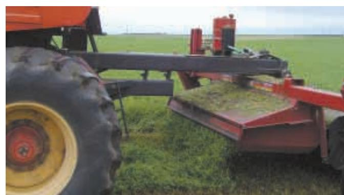
Machine articulates where the front mower's hydroswing tongue connects to an extended tongue on front of the combine. The cylinder on the tongue steers the machine.
