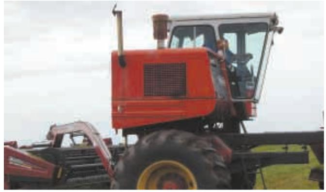
To make the power unit, he cut a Massey off behind the engine compartment and removed the rear wheels. The front mower mounts permanently to the combine, serving as the rig's front axle.
