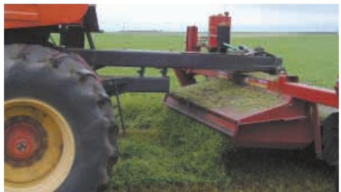
Machine articulates where the front mower's hydroswing tongue connects to an extended tongue on front of the combine. The cylinder on the tongue steers the machine.
