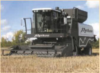
Rite Way Mfg, built 4 Pythons for sale this year. The combine replaces most belts and pulleys with individually controlled hydraulic motors.
