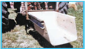
Merlyn Rieffer scored an old bathtub with an angle gr inder to cut it in two, then bolted scrap iron to the sides to mount it on a 3-pt. hitch.
