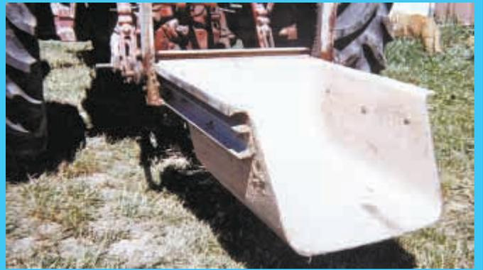
Merlyn Rieffer scored an old bathtub with an angle grinder to cut it in two, then bolted scrap iron to the sides to mount it on a 3-pt. hitch.
