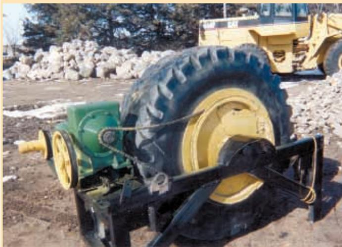
Prototype machine tumbles rocks inside a 25-in. tire. Inventor Don Emme sealed off the open sides of tire with steel plate. Since photo was taken he's put guards over chains.
