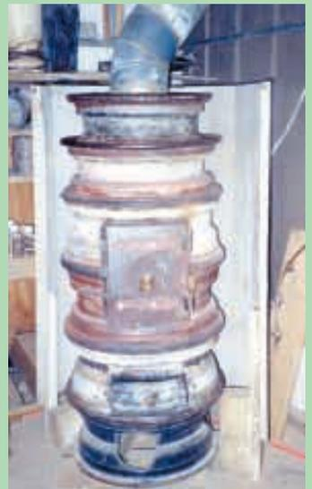
Howard Keele made this wood-burning stove by stacking six wheel rims on top of each other and then welding them together.
