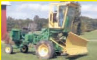
I turned a 55 Deere combine into a plow. We stripped off all the grain cleaning components. The engine's mounted at the back to counteract the weight of the plow up front. We also fitted it with a cab so we can work in comfort. Works very well.
