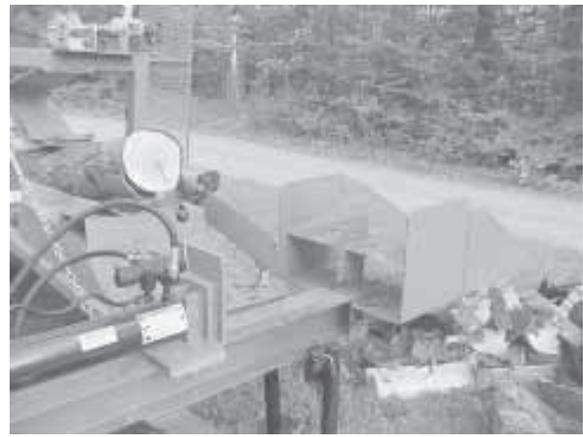
Cut log drops onto 4-way splitter.
