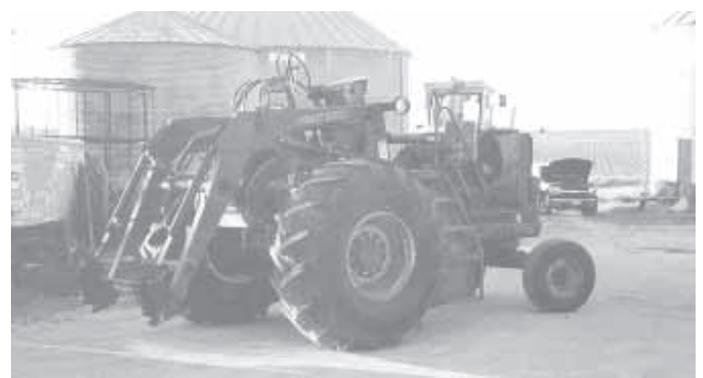
Schroeder converted an IH 815 combine. "The hydrostatic transmission on this combine connects directly to the engine so you can position the engine anywhere," he says.
