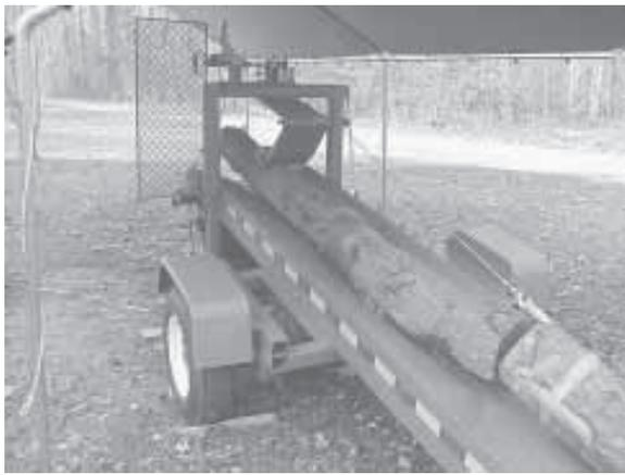
Winch pulls log onto splitting table where a chain saw is used to cut a 20-in. section.
