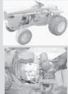
**Do-it-yourself conversion kits allow you to substitute Honda and Kohler engines for the original engines in Deere, Simplicity and Allis Chalmers garden tractors.**
