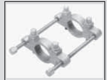
**Specialty designed puller grips both sides of the exhaust pipe joint. Turning the drive bolts separates the joint.**
