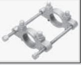
Specially designed puller grips both sides of the exhaust pipe joint. Turning the drive bolts separates the joint.
